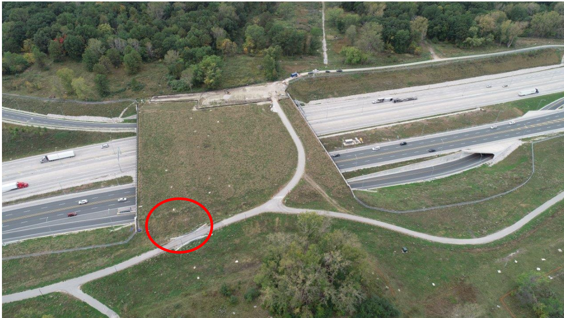
Figure 14: Aerial imagery of a wildlife overpass for snakes in Ontario showing a bike path and the location of an underpass on top of the overpass (red circle). The image also shows the vegetation on top of the overpass.
