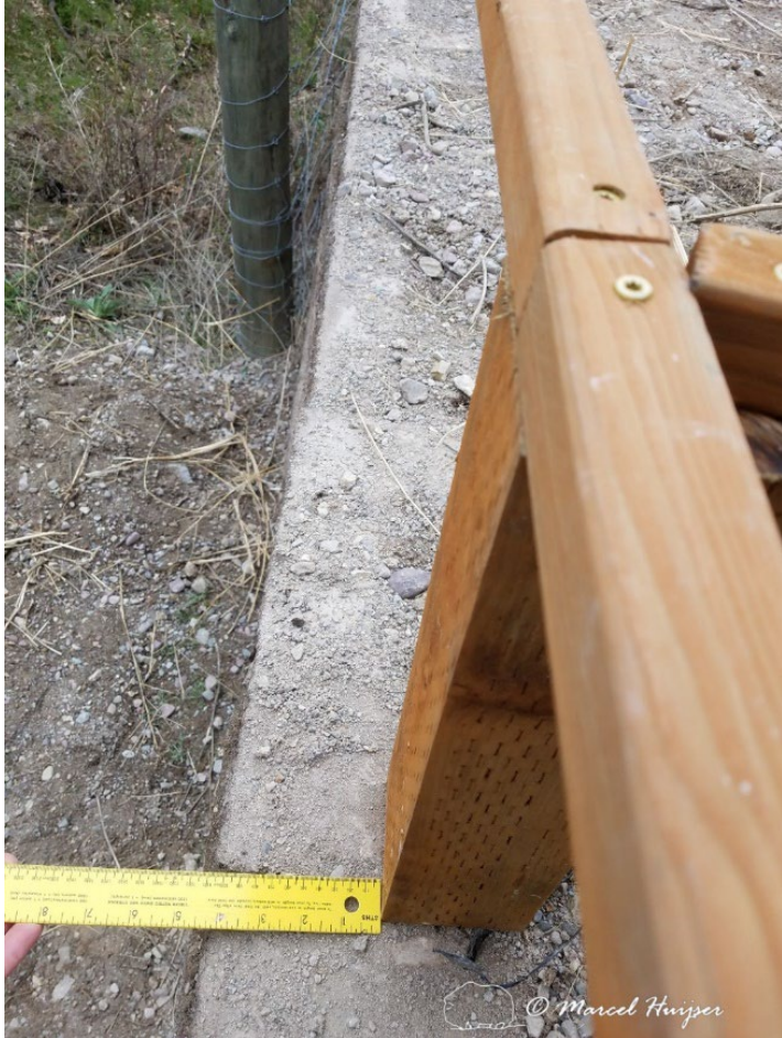
Figure 10: The wooden prototype had a setback of 10 cm (4 inches).
