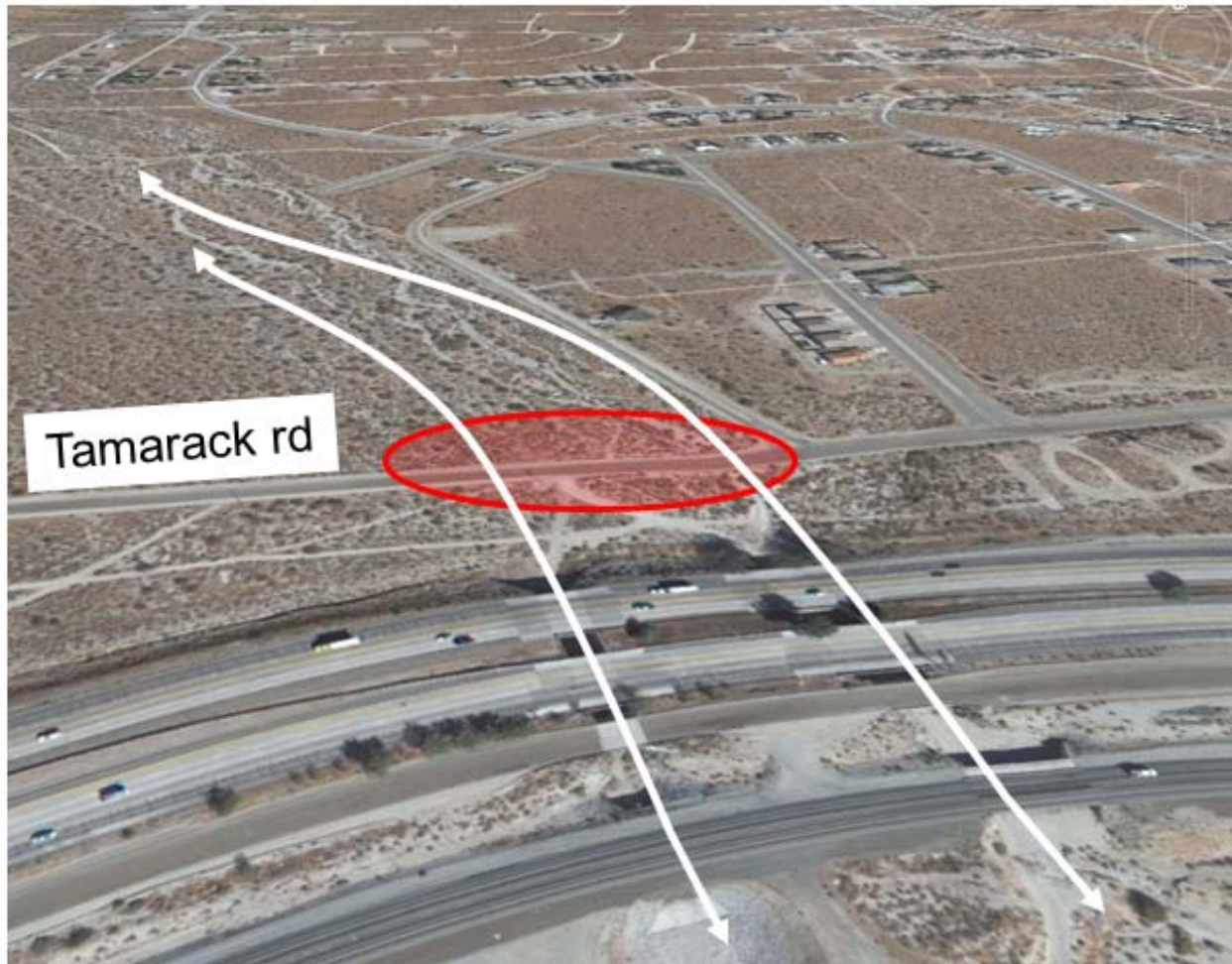
Figure 1.2: The existing bridges (east and west set) under the freeway (I-10), railroad, and southern frontage road on the east side of the Stubbe Canyon corridor. The red oval indicates the location of one or more proposed structures under the northern frontage road (Tamarack Rd). The white arrows indicate possible animal movements through the eastern and western set of crossing structures.
