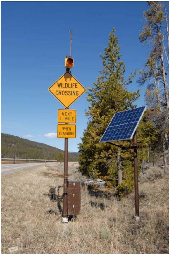
Figure 6. An animal detection system, designed to detect large mammals as they approach the road, and associated warning signs for drivers (© Marcel Huijser).
